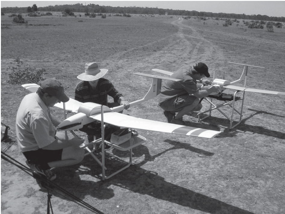
FIGURE 4. The Codarra Avatar was fitted with a HP IPAQ running a JACK agent connected serially between the radio modem and the flight control system. The agent provide autonomous control of the UAV: monitoring the aircraft state via the data sampled from the flight control system and controlling the aircraft through waypoints fed into the flight control system.
